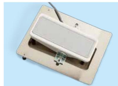
One-shot operation pedal is adopted to start the sewing machine. The sewing step is moved forward by depressing the front part of pedal, and it is moved backward by depressing the rear part of pedal.
